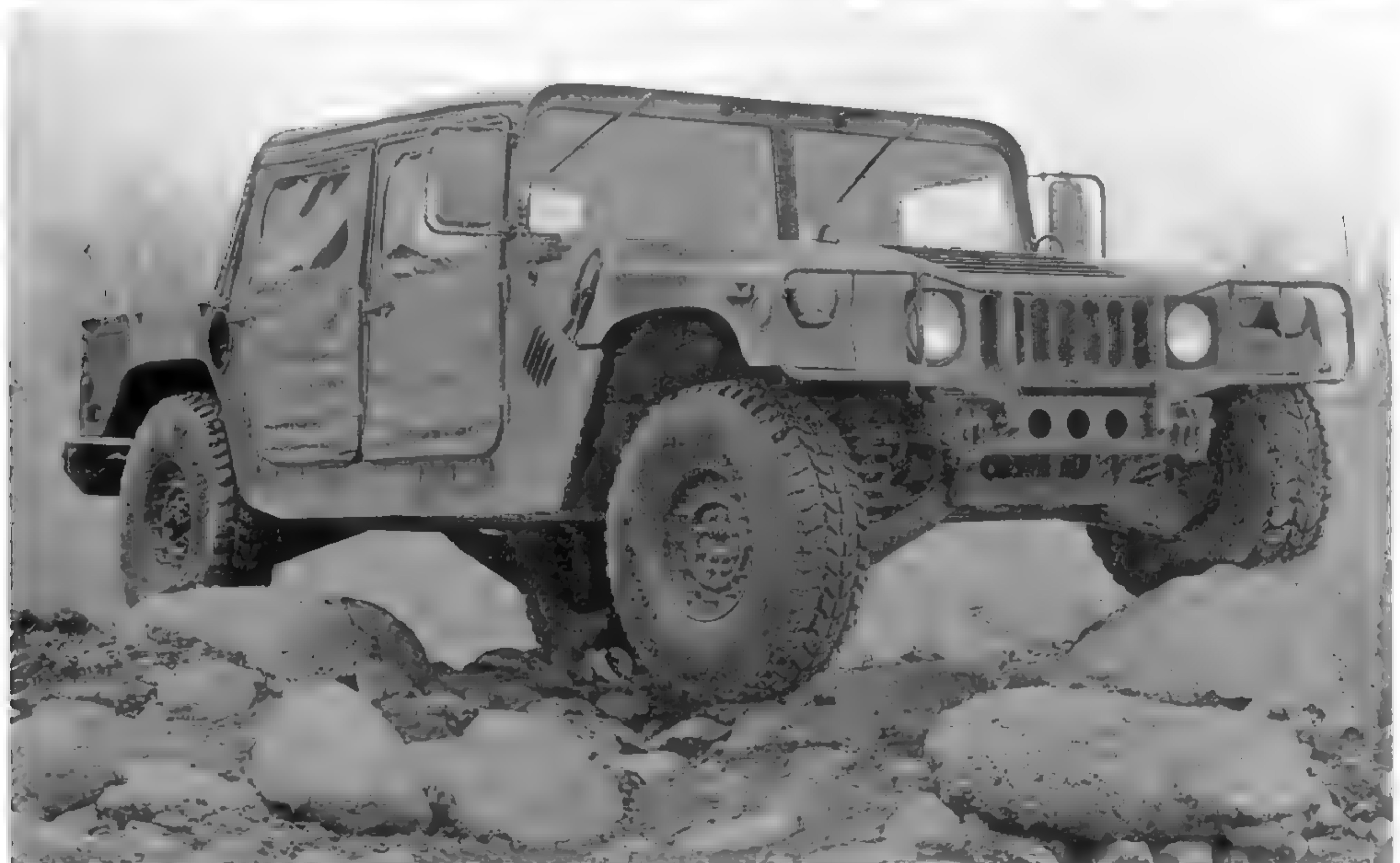
The M998 is the base vehicle of the HMMWV series. This one is configured as a four-man troop carrier with a soft-top enclosure. (Photo courtesy of AM General Corp.)
